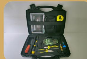
**Arson Investigation Kit**: Combustible hydrocarbons/ gas detectors detection plays important roles in suspected arson or fire scene. Kit detects acetylene, methyl chloride, iso-butane, acetone etc if present at the crime scene.
